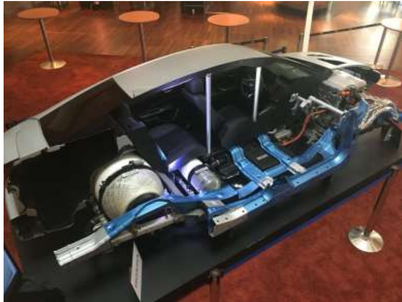
Hydrogen Powered: The major components of the Toyota Mirai, a hydrogen-powered car
