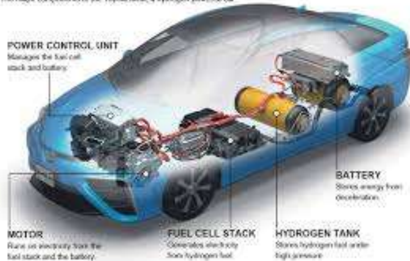
Hydrogen Powered: The major components of the Toyota Mirai, a hydrogen-powered car
